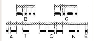
Diagram illustrating relative lengths of dashes and spaces referred to the duration of a dot. A dash is exactly equal in duration to three dots; spaces between parts of a letter equal one dot; those between letters, three dots; space between words, five dots. Note that a slight increase between two parts of a letter will make it sound like two letters.
