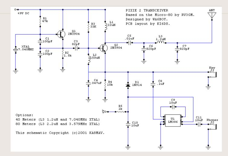
Shows how to build a radio from components.
